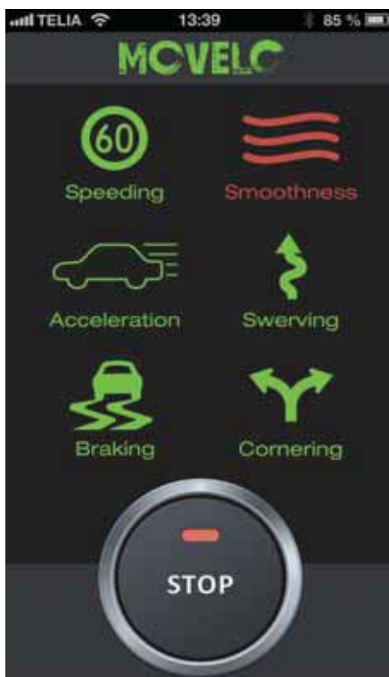
Fig 2. Example of insurance telematics user interface mimicking the vehicle dashboard. It provides real-time feedback to the driver [courtesy of Movelo AB].
