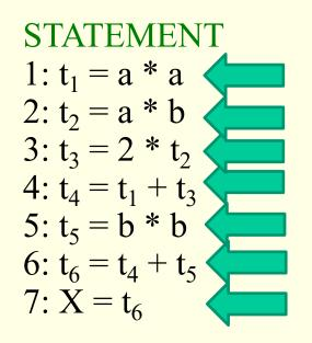
7: no temporary is live 6:  $t_6$ :use(7),  $t_4 t_5$  not live 5:  $t_5$ :use(6) 4:  $t_4$ :use(6),  $t_1 t_3$  not live 3:  $t_3$ :use(4),  $t_2$  not live 2:  $t_2$ :use(3) 1:  $t_1$ :use(4)
